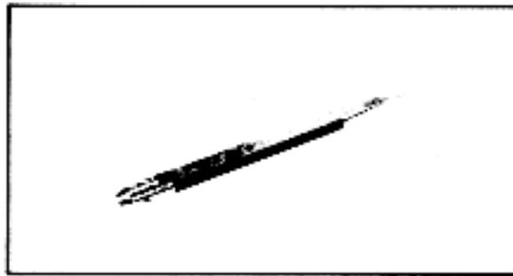
FIGURE A9. BOLT CATCH PIVOT PIN PUNCH (P/N 62680) (SEE FIG. 3-3K, PAGE 28)
